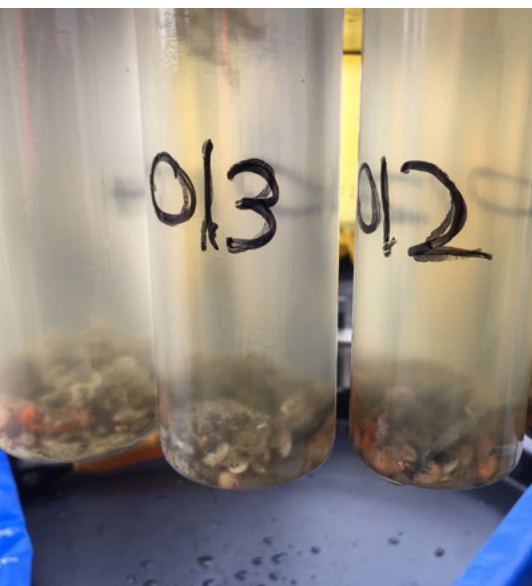
Close-up of McLane Sediment Trap collection cups post recovery.
