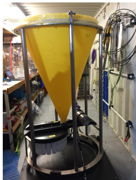
SAZ McLane Sediment Trap assembly prior to deployment.
