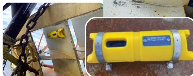
Moana sensor attached to trawl door using tough jacket #3 and brackets.
