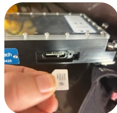
Insertion of a SIM card in the deck unit.
