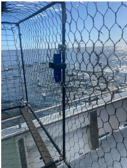
Figure 2. Temperature and pressure (TP) sensor (Moana) attached to fish trap.
