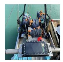
For low latitudes (less than  $\sim\!25$  degree), to prevent overheating, the deck unit should be installed at a 45° angle.
