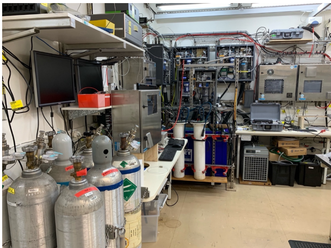
Figure 1 Test and calibration facility for f\text{CO}_2 system pre-deployment checks
