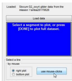
Figure 8 Control panel for line selection by mouse.
