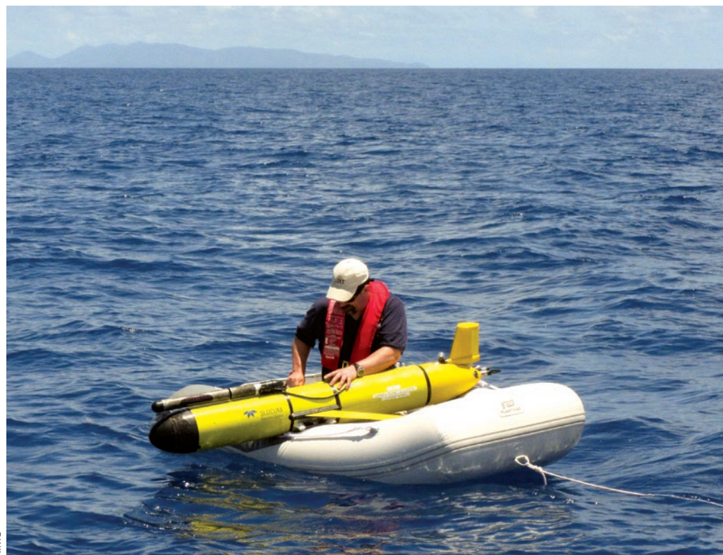
Rob Gregor from CSIRO making final adjustments to the ballast of a slocum glider before a deployment on the Great Barrier Reef.
