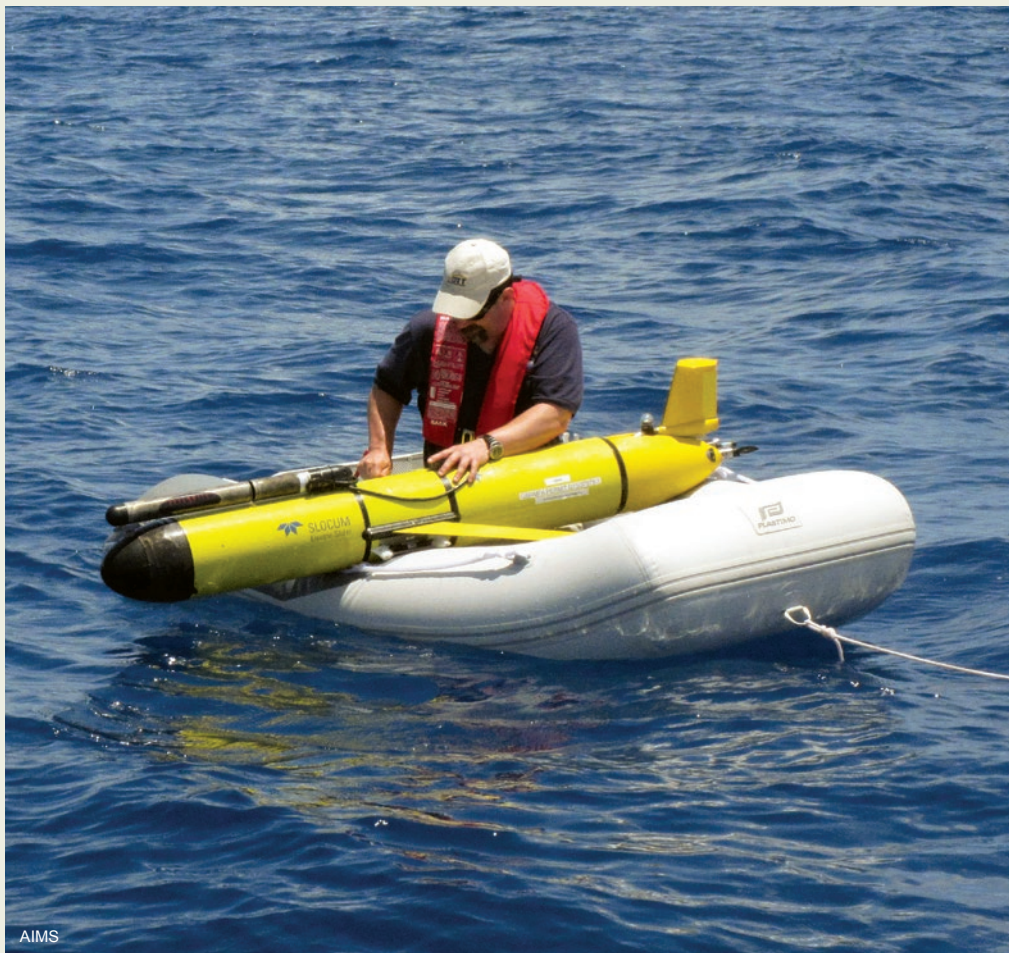
Rob Gregor from CSIRO making final adjustments to the ballast of the Slocum glider.
