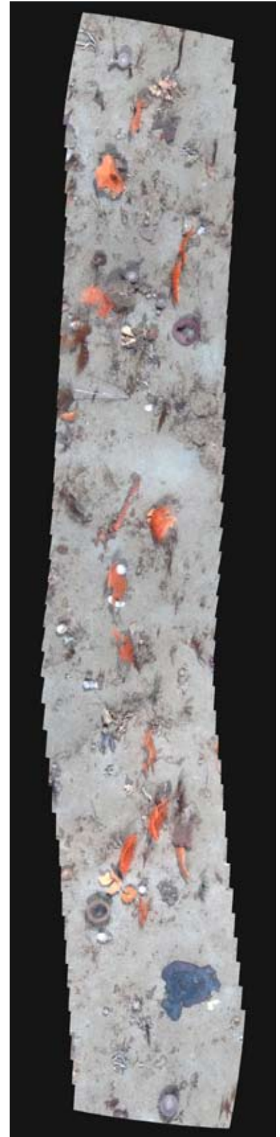
A sample mosaic from the Autonomous Underwater Vehicle (AUV) taken at Ningaloo marine park, Western Australia showing sponge beds in 80m of water. The AUV was maintaining an altitude of 2m, giving a 1.5m swath, and traveling at 0.5m/s. The mosaic is composed of 40 images captured at 2Hz and represents a 10m transect.
