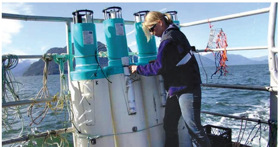
Heidi Lydersen of the Pacific Ocean Shelf Tracking (POST) project – a North America based tracking program that helped pave the way for AATAMS – prepares some VR3 receivers (encased in the aqua tubing near the top) to be deployed. (Photo courtesy of POST).
