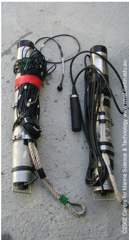
Underwater Sound Recorders that will be used in the Acoustic moorings. Photo courtesy of Rob McCauley.
