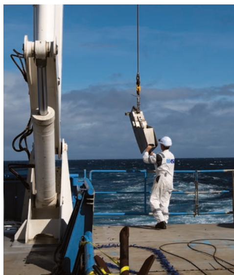
Above: A member of the ship's crew deploying the IMOS CPR. Right: Stephen Thomas of the MNF with the IMOS In Situ SST Autonomous Radiometer that measures sea surface temperature.
