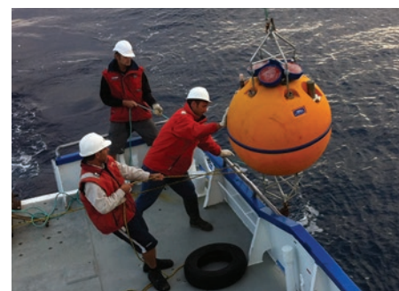
Oceanographic mooring being deployed at the SA-IMOS Kangaroo Island National Reference station. Observations provided by IMOS are essential to the development of the hydrodynamic model used to simulate larval transport and settlement.
