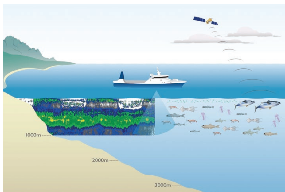
This figure demonstrates how bioacoustics data is collected by transmitting a pulse of sound in the water that reflects off the species to produce an echogram.
