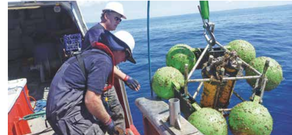
NRS team recovering subsurface instrument arrangement.
