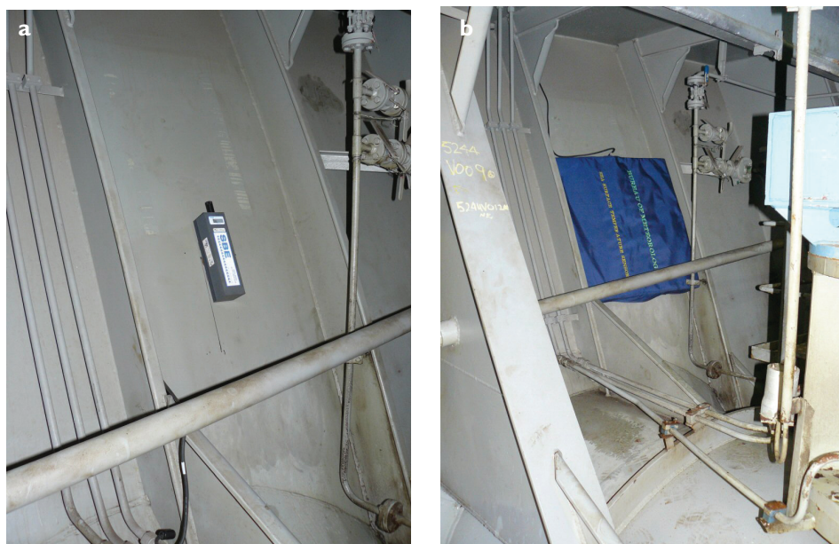
Fig 4: The Sea Bird SBE 48 hull contact temperature sensor (a) installed against the exterior hull of the PV Spirit of Tasmania II in the bow thruster room, and (b) covered with the custom-made insulating pad
