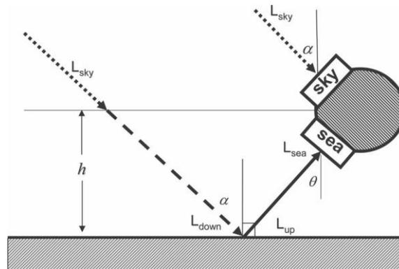
Figure 4: Geometrical set up of the ISAR on RV Investigator (Figure taken from Donlon et al., 2008). In this case the nadir viewing angle,  $\theta$ , is  $25^\circ$  and the height,  $h$ , above the ocean surface is typically  $\sim 19.6$  m.
