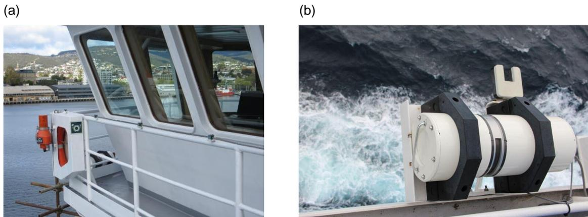
Figure 3: Photos of the ISAR instrument as installed on RV Investigator, showing (a) view from port-side bridge deck during installation, and (b) view from above at sea.
