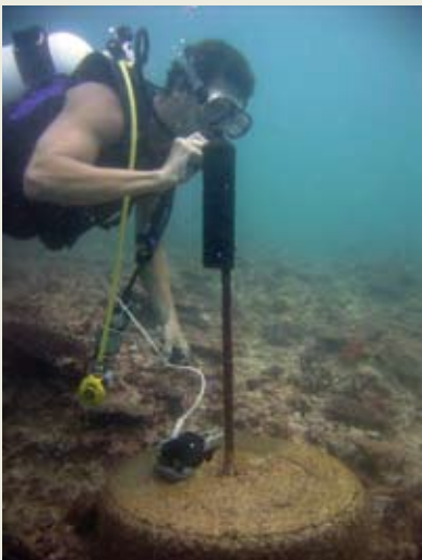
Dr Charlie Huveneers, the AATAMS Technical Officer, deploying an acoustic receiver at Ningaloo Reef, WA. Photo courtesy of Frazer McGregor.
