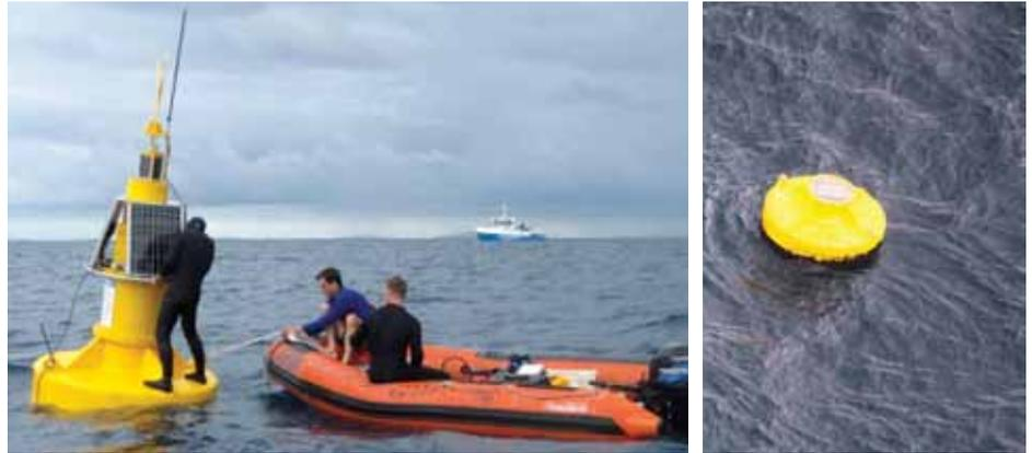
A wireless sensor float being deployed at Rib reef in 2010 (left). The damage caused by Cyclone Yasi as it went through, the top section of this float has been completely ripped off (right).
