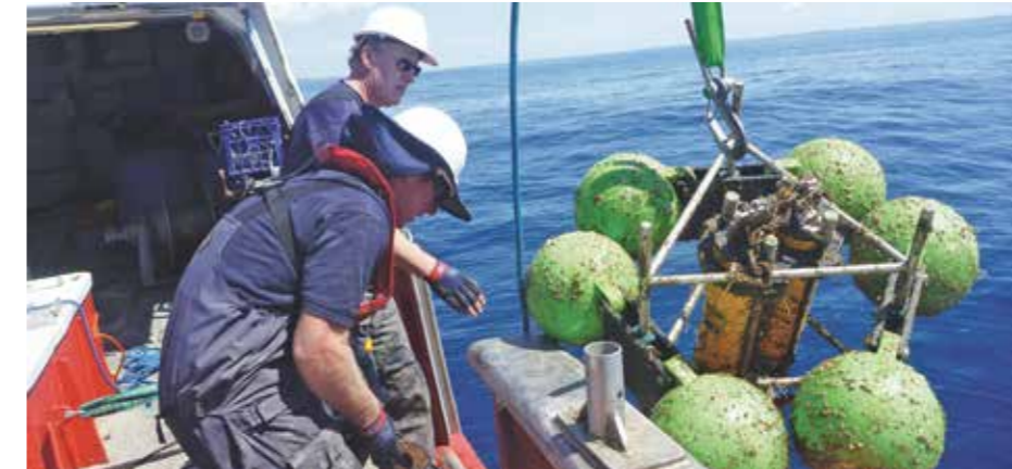
NRS team recovering subsurface instrument arrangement.
