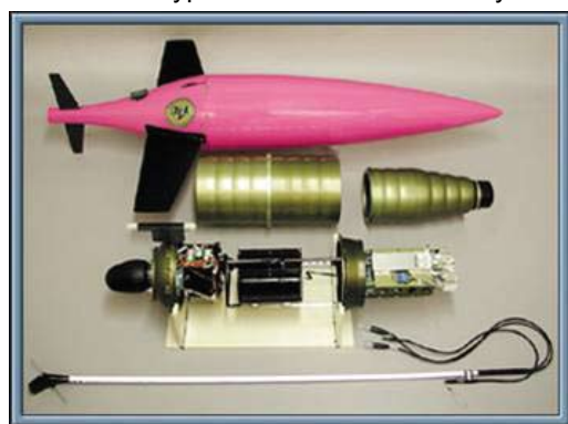
Figure 2. Inside a Seaglider.
