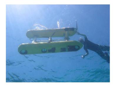
The ocean going AUV 'Sirius' is managed by the University of Sydney's Australian Centre for Field Robotics (ACFR). Sirius is specifically designed for undertaking high-resolution benthic optical and acoustic imaging work and is equipped with a full suite of oceanographic instruments.
