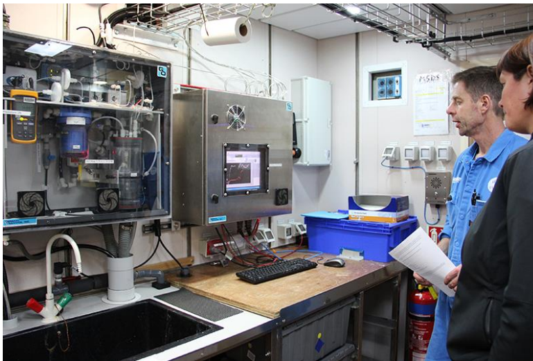
Stephen Thomas (MNF) shows Marian Wiltshire (IMOS) the pCO 2 equipment in the underway lab on the RV Investigator
