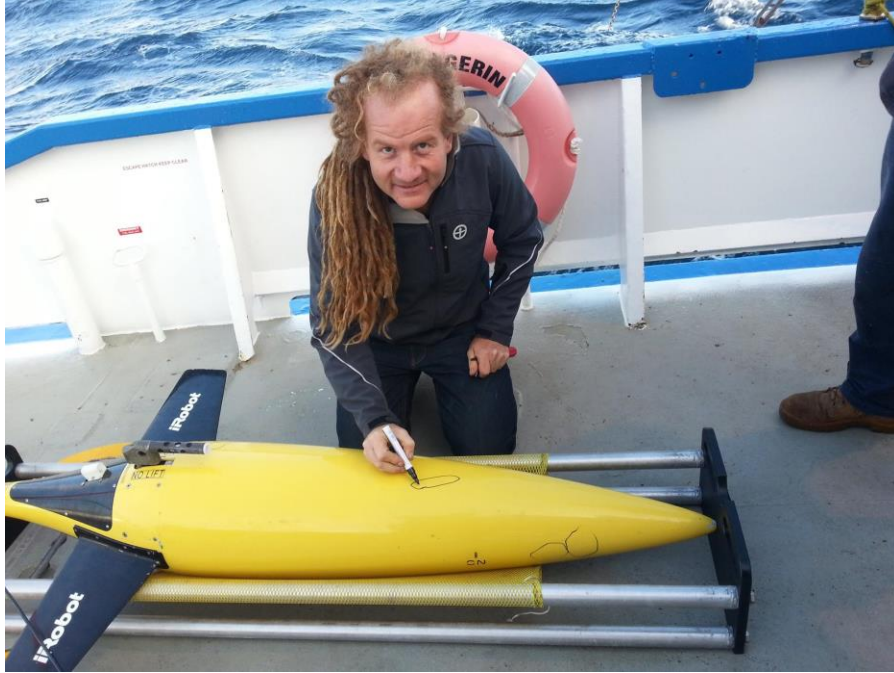
Ocean glider recovered after South Australian mission. Dennis Stanley (UWA) shows evidence of shark bite
