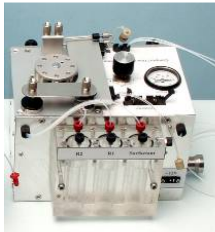
Fig. 3. Flow-analysis instrument configured for phosphorus determination (Water Studies Centre, Monash University). The dimensions of this instrument are such that it would comfortably fit into a shoebox. This example has been operated in underway mode in the Victorian 'Two Bays' Study (Pelican Foundation), and it is soon to be deployed for a proving voyage across Bass Strait on a 'Spirit of Tasmania' ferry (joint Monash University – Vic EPA project).
