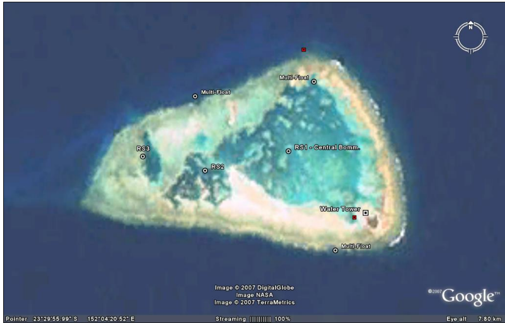
Figure Thirteen: Proposed locations of the One-Tree Island equipment – key: RS = Relay Spar, Multi-Float = Multi-Float Buoy, red squares are \mu Node floats. Water Tower is the base station on the Island.
