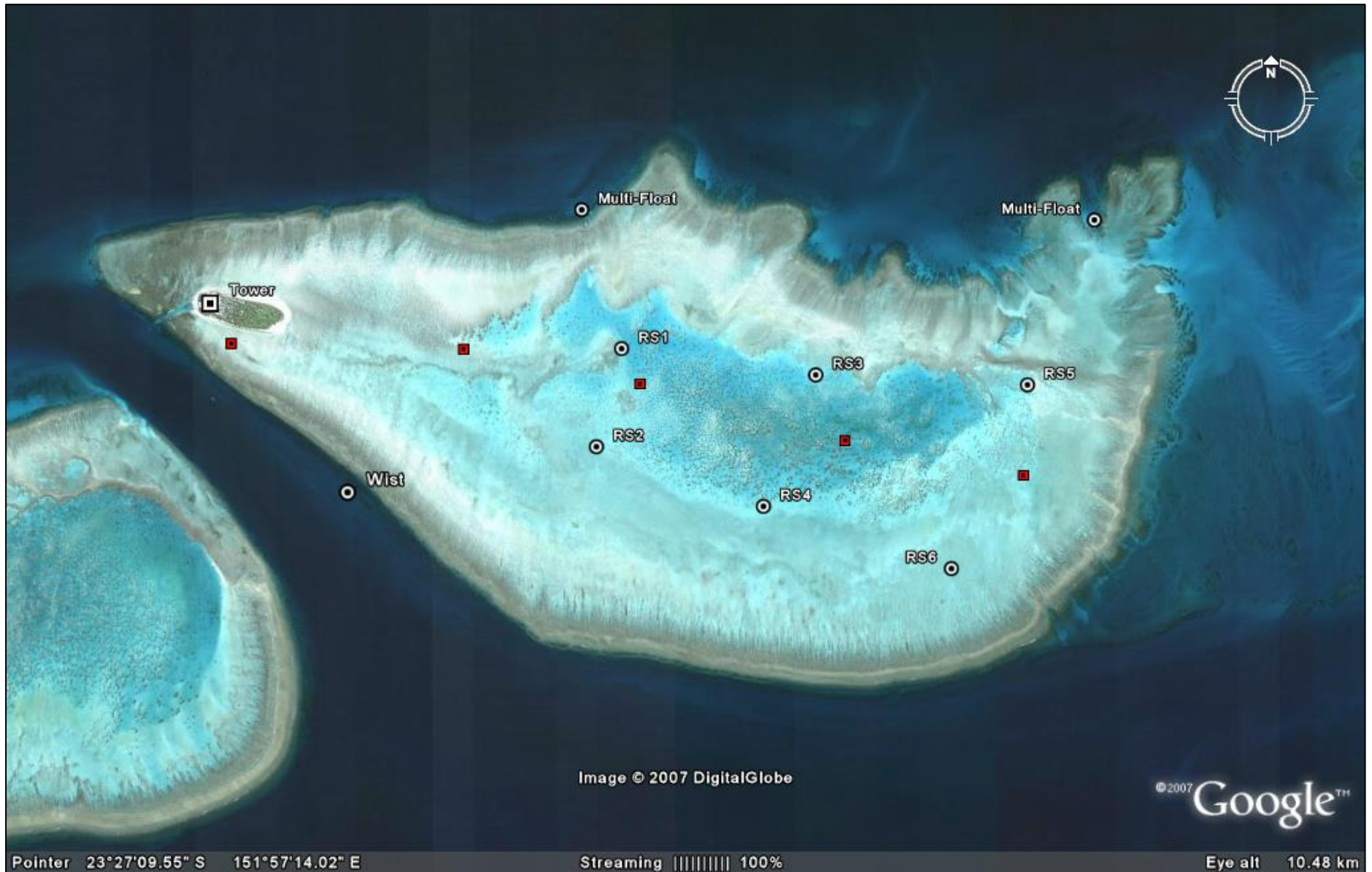
Figure Twelve: Proposed locations of the Heron Island equipment – key: RS = Relay Spar, Multi-Float = Multi-Float Buoy, red squares are \mu Node floats. Wist = Wistari Channel Multi-Float(s), Tower is the base station on the Island.
