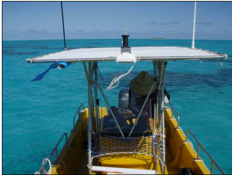
Figure Six: Boat mounted mobile station, aerial is the black unit to the top left of the photograph.
