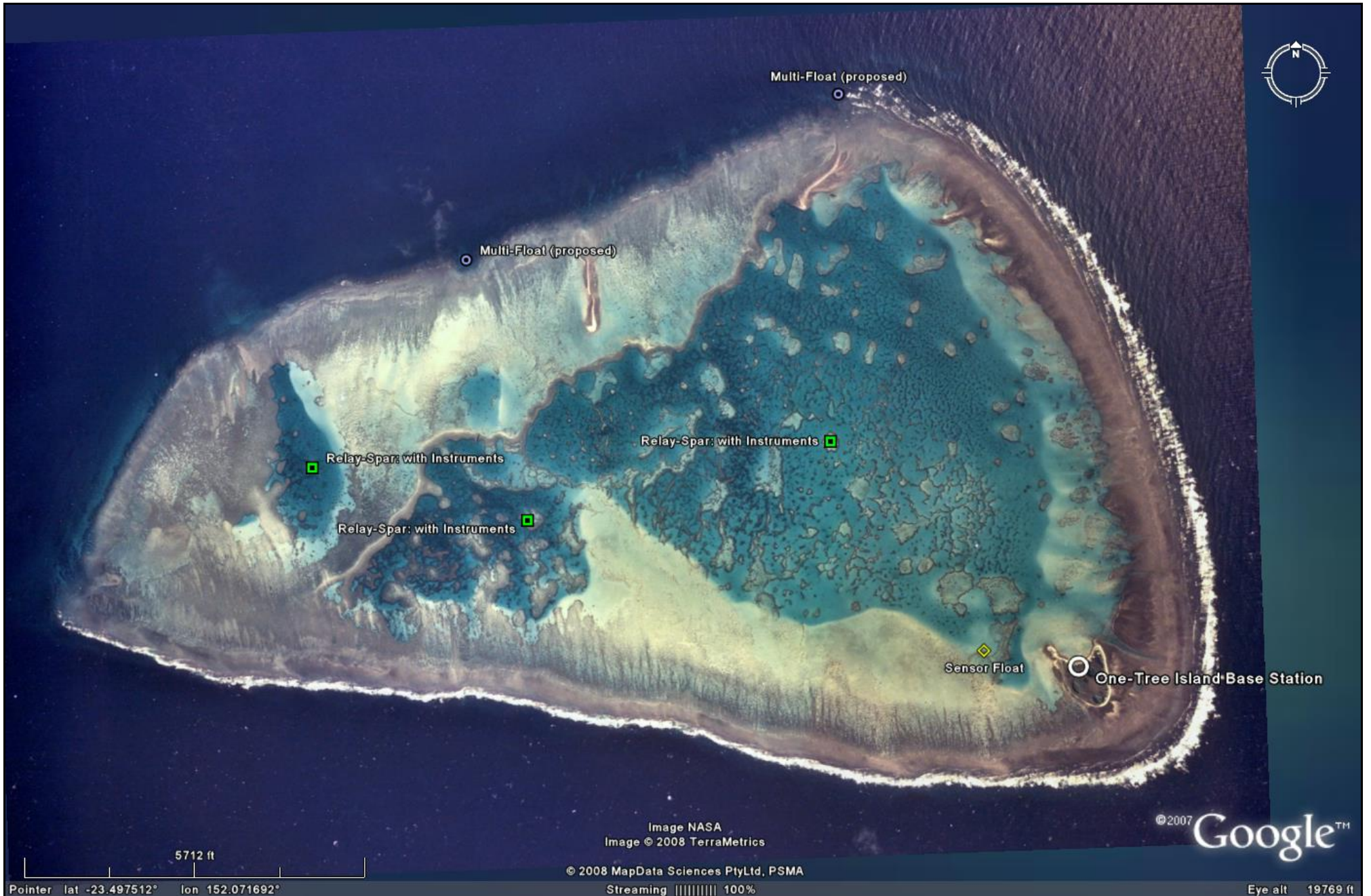
Figure Two. Planned Deployments for One-Tree Island. Initial deployment will include the base station and three relay-poles with sensors, multi-float buoys will be deployed on subsequent visits.
